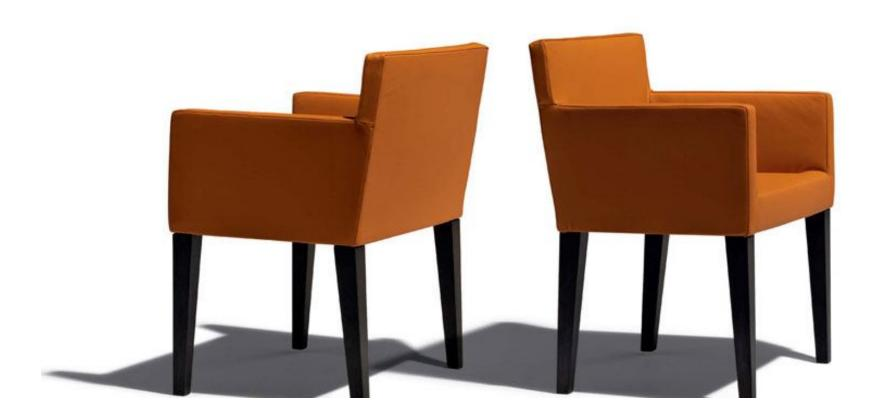
Armhair with welded steel frame reinforced with webbing on seat and back injected moulded polyurethane foam with a density of 65/75 kg/m³. Legs in oak wood fixed to the structure by stainless steel bolts. High resistance lacquer.
