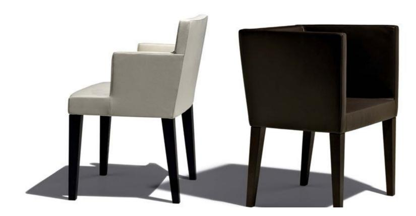
Armchair with welded steel frame reinforced with webbing on seat and back, injected moulded polyurethane foam with a density of 65/75 kg/m<sup>3</sup>. Legs in oak wood fixed to the structure by stainless steel bolts. High resistance lacquer.
