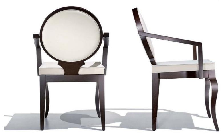
Chair with ash frame with mortise joints, backrest made of curved slats of ash, seat padded with 40 kg/m³ density polyurethane foam. Seat panel made of birch plywood with high resistance paint finish.
