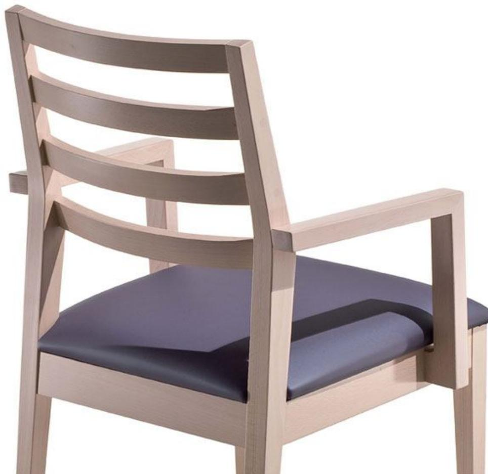
Armchair with ash frame with mortise joints, backrest made of curved slats of ash, seat padded with 40 kg/m<sup>3</sup> density polyurethane foam. Seat panel made of birch plywood with high resistance paint finish.
